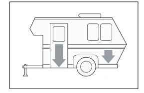
total cargo weight should be positioned in the front portion of the trailer and 40% in the back. Then, the load should be adjusted until the proper tongue/king pin load ratio is achieved.
