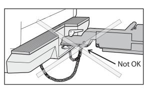
binding; however, note that excessive slack will allow the chains/cables to drag on the ground.
